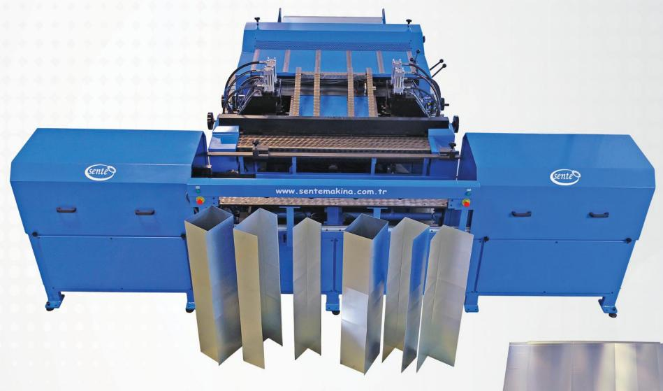
This machine and Auto Duct Forming Machine With Notchers has the same characteristics in addition to it's cassette system. It is a very helpful machine in order to produce TDF/TDC self flanged duct as it makes C and P notches to make the sheet metal ready to be feed to TDF/TDC flange forming machine. Also it eliminates the need for a lock forming machine as it makes pitsburgh's male and female which decreases production time and effort and increases your profit.
