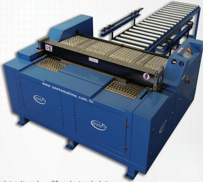
This machine is designed to produce self flanged rectangular ducts with TDF flange.
