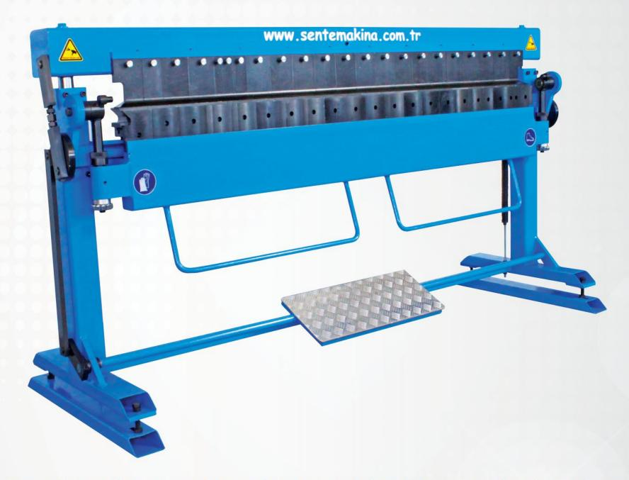
With its strong welded steel frame this machine can fold sheets made from different materials such as galvanized steel, aluminum, zinc and stainless steel. Also duo to its diffirent sized segmented blades, it could easily fold different sized boxes.
