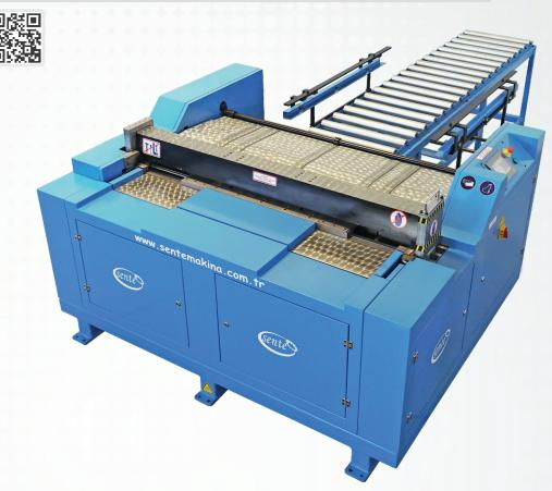
The Automatic Flanged Square Channel Bending Sealing Machine is utilized to transform products into square channels by bending the pre-flanged edges and sealing Pittsburgh seams. Its primary design objective is to manufacture self-flanged rectangular ducts with TDF flanges.
