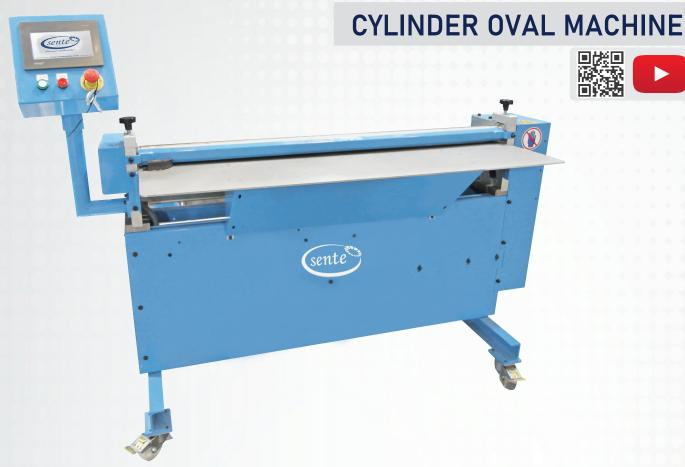
This machine is designed to produce oval channel fitting segments by bending sheet metal sheets between cylinders. It boasts PLC control, enabling seamless automation of all operations based on the data input through the screen. When the minor and major measurements of the oval canal are entered, the sheet metal opening dimensions are automatically calculated and projected on the screen. This process eliminates the possibility of errors in calculations that an operator might make.
