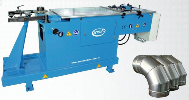
This machine is designed to assemble round cross-section segments, obtained by cutting on a plasma cutting machine, into a complete ductwork system. The machine comprises two stations: the first station opens male and female flange locations for the segments, while the assembly and closing process is carried out at the second station.
