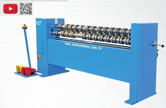
The Fittings Rounder is an invaluable machine used to round both the inside and outside parts of air duct elbows. Its sliding rollers allow pre-seamed parts to be rounded without closing their seams.
