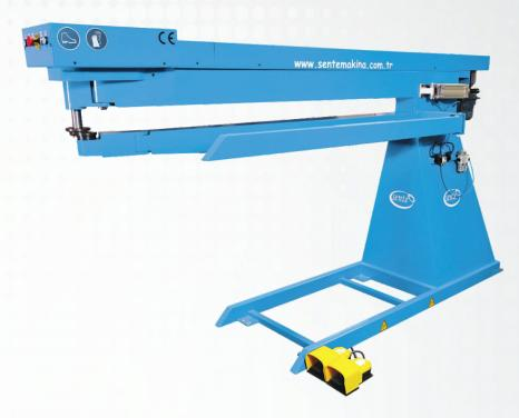
The Square Elbow Closing Machine is specifically designed for securely sealing the Pittsburgh seams of elbows and straight channels. Widely employed in ductwork applications, particularly in HVAC systems, this machine offers a straightforward and efficient operation. Positioned along the edges of the channel, it facilitates connections by compressing the clamps in place.
