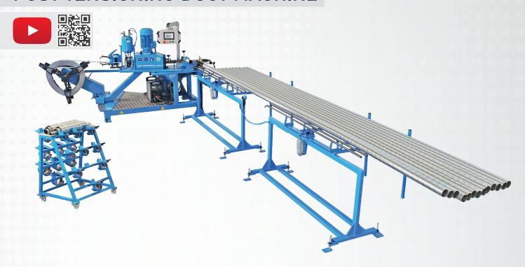
This machine is designed to produce flexible pipes used in the construction industry, which create spaces under concrete. The grooves on the pipe enhance its resistance to crushing. Thanks to the flexibility of these pipes, there's no need for additional equipment like elbows.
