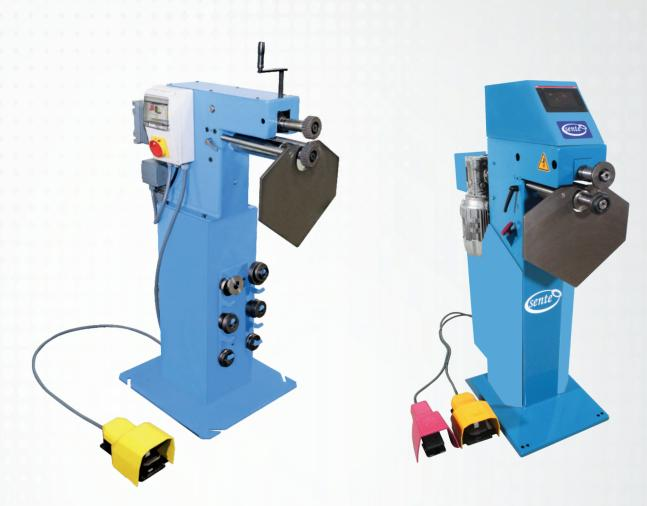
Swaging machine is multi-purpose machine built to shape the edges of air ducts and fittings pieces
