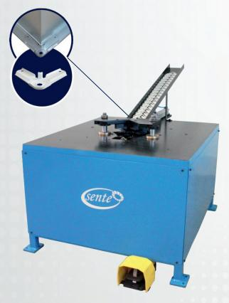
This machine is designed to attach the necessary corner apparatus to TDF Self-flanged channels using bolts. The machine automates the corner feeding process through a built-in corner hopper, resulting in swift and secure fastening. This automation eliminates the need for manual intervention by the operator, ensuring a safe working environment.
