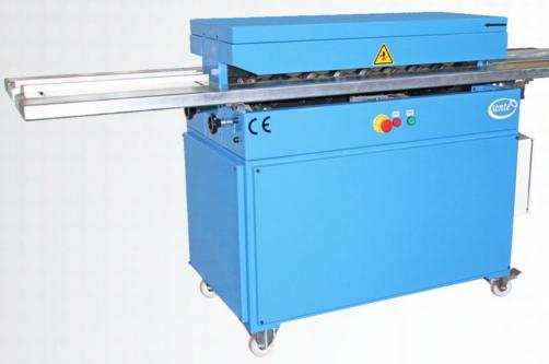
It has got 9 stations. Machine can work with up to 1,2 mm sheet thickness. Two roller sets are standard in the machine. One side can be Pittsburgh and the other side can be Snaplock. Roller sets are made of high quality steel in order to extend its life time. Working height can be adjusted in order to increase the safety. It works very quite. Also sheet's radius could be changed with its adjustable roller set.
