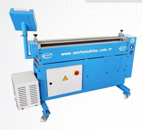
Cylinder Oval Machine is a machine to roll the sheet according to entered oval size on PLC screen. Oval Roller Machine rolls oval elbow, oval reducer and T-pieces parts which are necesary for oval duct systems.
