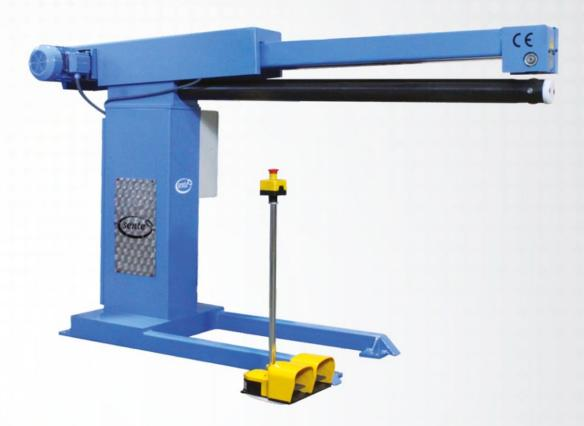
The Lock Seam Closing Machine, makes the seam within seconds for both the outside and inside positions. It is possible to make ducts with diameters from 100 mm to 1000 mm. By turning the channel, the working length can be doubled. channels. It saves labor costs and time with its fast working capacity.
