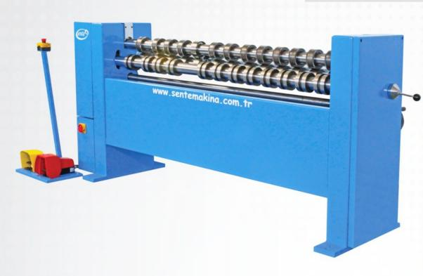
Fittings Rounder is a very useful machine used to round the inside and the outside parts of air duct's elbow. It's sliding rollers allows pre-seamed parts to be rounded without closing thier seams.
