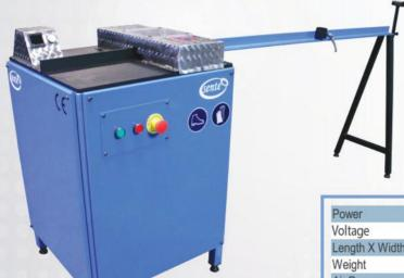
This machine is used for flange cutting. It cuts the flanges according to desired lenght. It makes precise and burr-free cutting with the 1500 mm measure ruler. This is a very useful machine with the number counter. Machine gives an automatic light signal when the requested job is done.
