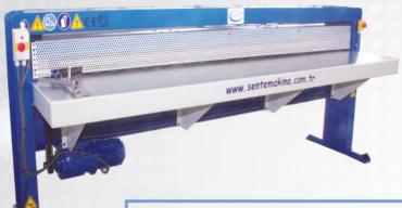
This machine allows you to make a reinforcement for the ducts. It is very easy to use. You can use this machine in order to make Z design, Trapezoid design or U bead form.
