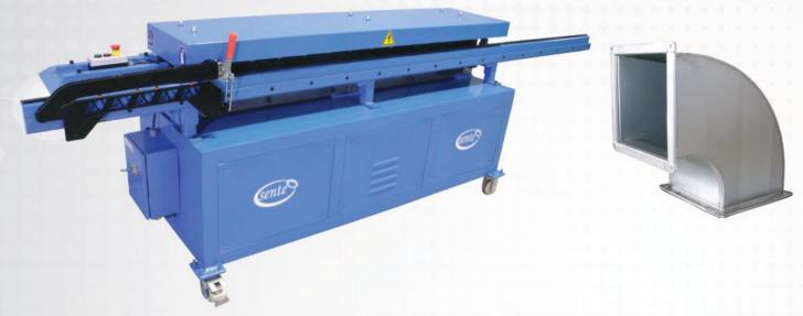
This machine allows you produce your fittings with TDF flange system. No need to insert extra flange after you compose your fittings. There are two roller sets on the machine. One side form the flange, and the other side form the clip which will be neccesary for connection between two ducts.
