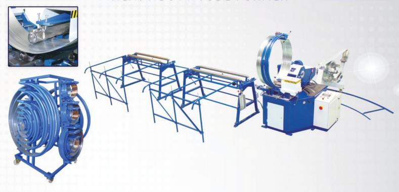
Heavy duty tube former machine is designed to produce ducts in desired diameter and length. Machine is designed to fulfill the Eurovent and Smacna standards. It allows you to manufacture high quality ducts in a short time with quite operation. The outstanding slitter cuts the spiral ducts without noise or hot sparks as known from the saw and provides smooth tube ends without debarring.
