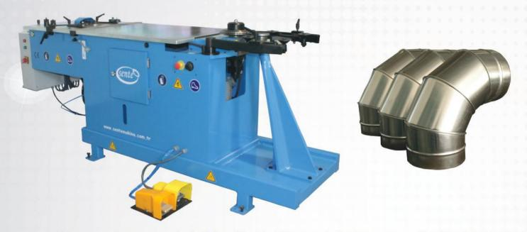
This machine allows you to make the fittings (elbows) which you cut in the plasma cutter machine. By using this machine you can save time and man power up to %80. It allows you to use 1,2 mm. thickness of sheet in order to make fittings, reductions and end plates.
