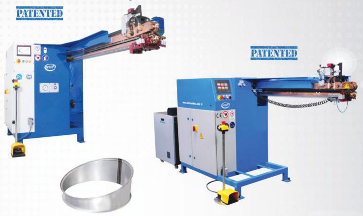
This machine allows you to weld the straight and circular sheets without burning. This operation is made by the copper wire. This machine decreases your labour cost and saves you money. As it is a fully automatic machine, it is very easy to use.
