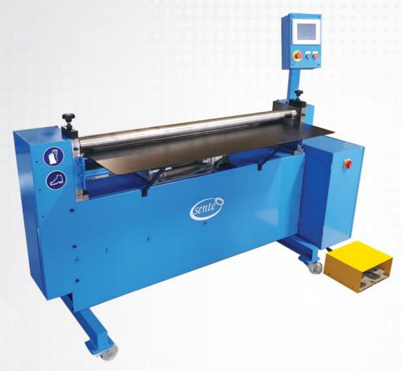
With this machine a straight sheet is turned into oval shape by passing through cylinders. With the help of PLC control the machine is automatically adjusted according to the dimensions entered from the screen. Sheet's flaten dimensions are automatically measured according to the wanted oval major and minor dimensions so the human calculation error is removed.
